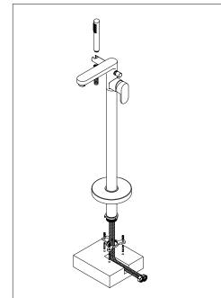
Please check that your pressure is suitable for this product before installation, details can be found on our website, recommed minimum working pressure: 0.5 bar, maximum working pressure: 3 bar
